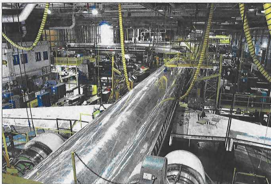
The pulse line acts as the heartbeat of the Tulsa facility, reducing the number of mechanics needed for heavy C-checks.
