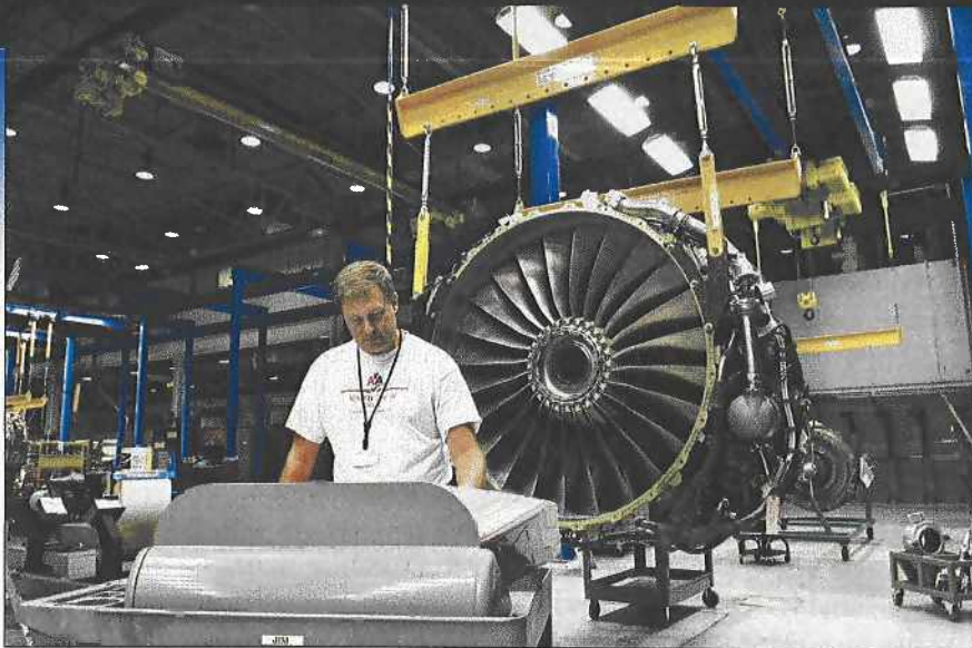
A mechanic is shown in the U-shaped gantry area, a space designed for efficient engine overhauls.
