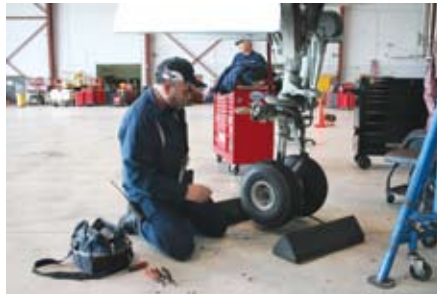
Eagle AMT, Tim Griffin services the nose gear strut on a Saab 340
